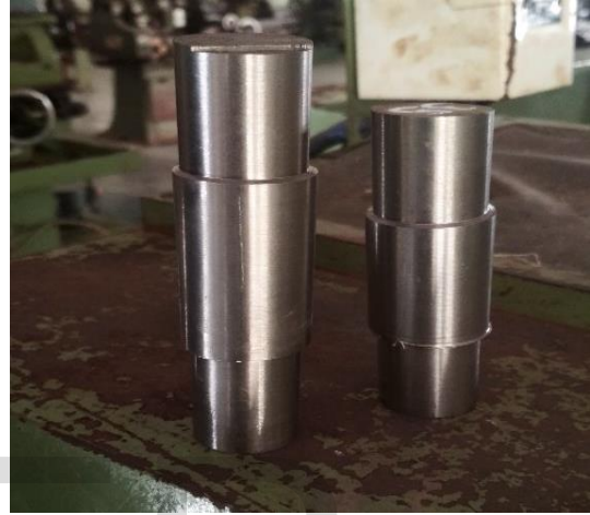
Fig.3. Titanium Grade 2 (after turning process)
